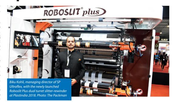
The ramp up and ramp down time of Roboslit Plus has been reduced to 45 seconds. This allows converters to actually finish their job by running the machine at the maximum speed of 1000 m/minute even while working on short-run jobs, which may be as small as 800 meter.
